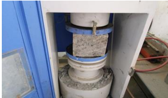
Figure 1: Compressive testing of concrete block
