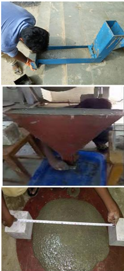
FIG. 1 TESTS ON SCC FOR WORKABILITY REQUIREMENTS AS PER EFNARC
