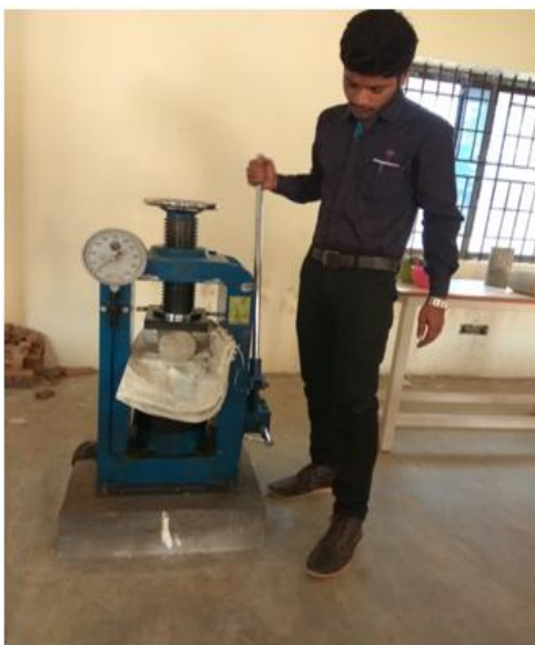
Fig 14: Split Tensile Strength test
