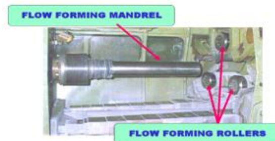
Fig 2.2: Arrangement of Mandrel & Rollers.
