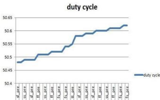
Fig. 6. PVT Corner Analysis of Duty Cycle
