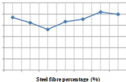
Fig. 6 Relationship between Cost/tensile strength and steel fibre percentage (%)
