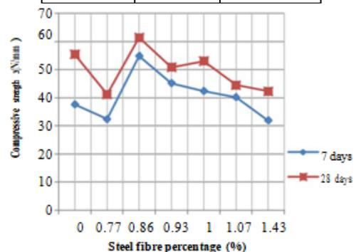
Fig. 4. Relationship between compressive strength (fcu) and steel fibre percentage (%)
