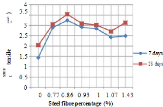
Fig. 5. Relationship between splitting tensile strength (fct) and steel fibre percentage (%)
