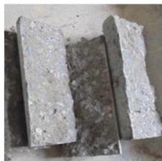
Fig. 10 Failure of plain concrete Cylinder
