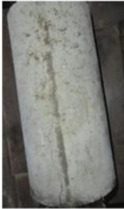
Fig. 11 Failure of SFRC Cylinder
