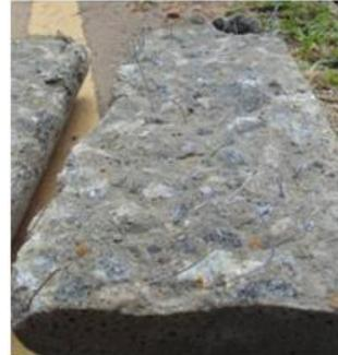
Fig. 7 Steel fibres distribution of cylinder specimen
