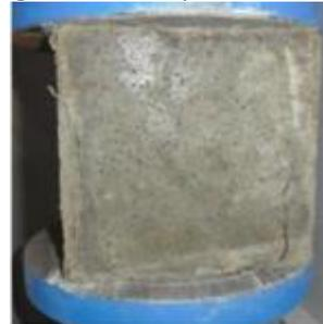
Fig. 9 Failure of SFRC Cube
