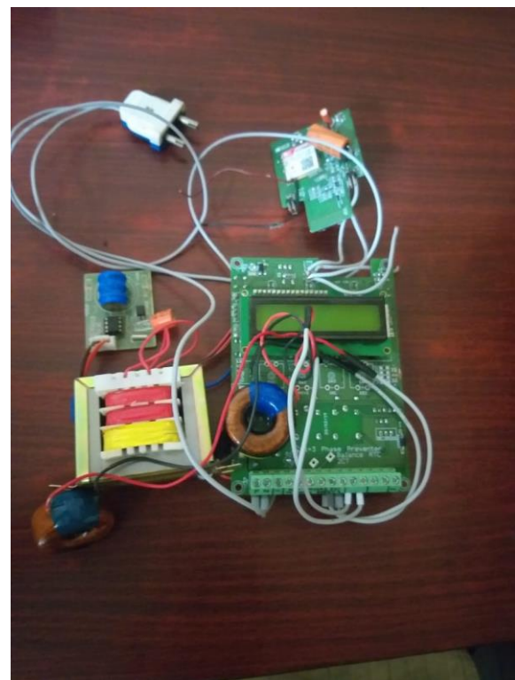
Figure.2: Prepaid Electricity meter system
