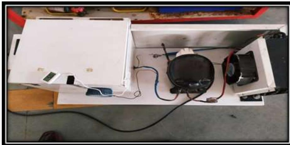
Figure 3 Fabricated model of VCR cycle
