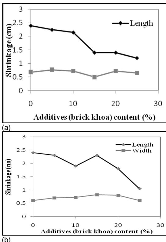
Figure 8 Variation of shrinkage with additives content at fourth day for (a) specimen 1 (b) specimen 2
