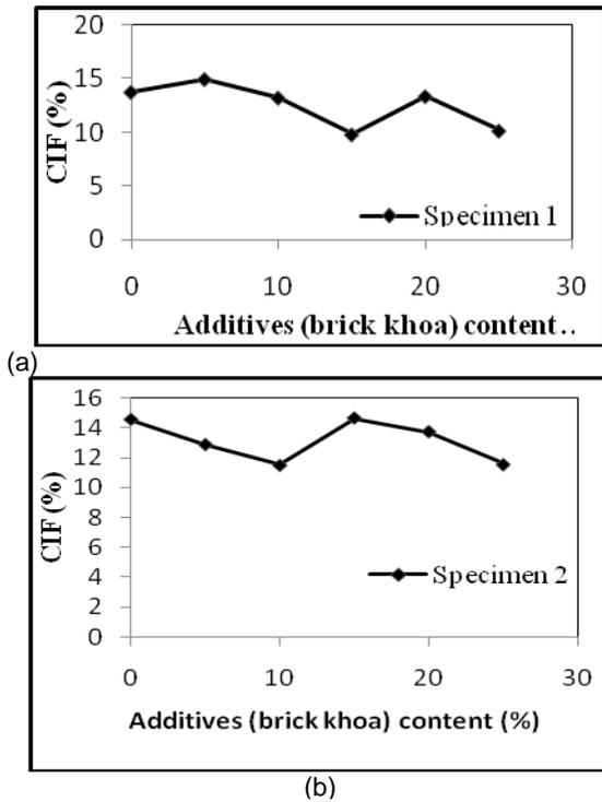
Figure 7 Variation of CIF with additives content at sixth day for (a) specimen 1 (b) specimen 2
