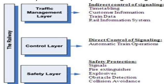
Fig 2. Schematic diagram of railway layers
