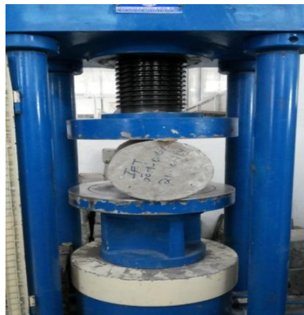
Fig 6: Tensile strength test on Concrete cylinders
