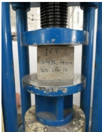
Fig 2: Compression test on Concrete cube
