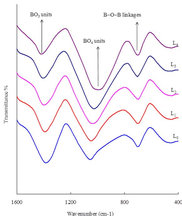
**Fig. 3** IR spectra of  $\text{Li}_2\text{O}-\text{Na}_2\text{O}-\text{B}_2\text{O}_3$  doped with MnO glasses
