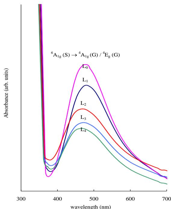
Fig. 1 Optical absorption spectra of  $\text{Li}_2\text{O}-\text{Na}_2\text{O}-\text{B}_2\text{O}_3$  doped with MnO glasses
