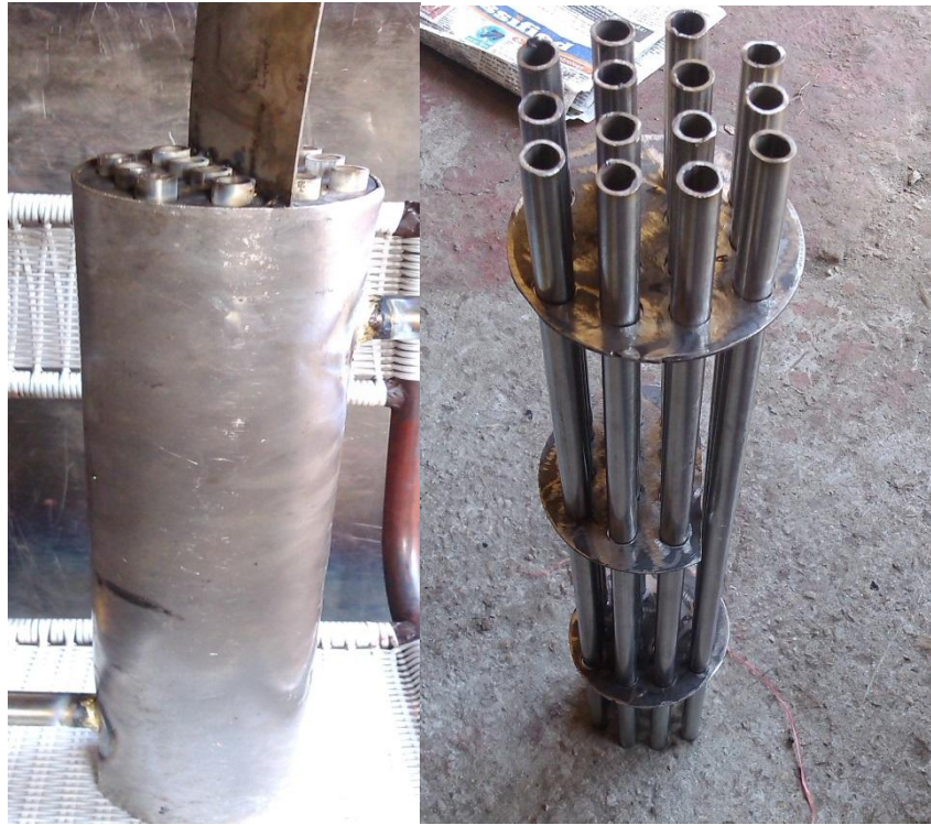
Fig 2: A view of condenser
