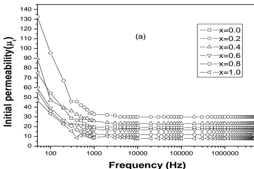
**Fig.2.** Frequency dependence of initial permeability ( $\mu_i$ ) for Zn substituted  $\text{Li}_{0.5x/2}\text{Zn}_x\text{Fe}_{2.5-x/2}\text{O}_4$  sintered at  $500^\circ\text{C}$ .
