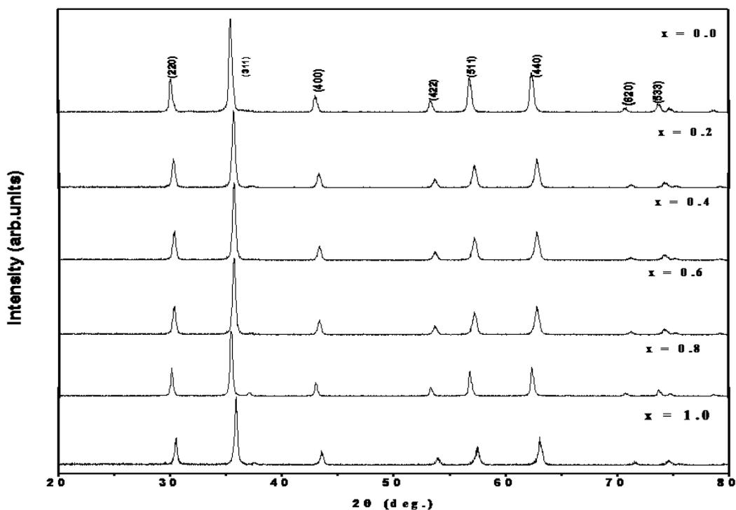
Fig. 1 Room temperature XRD pattern of Li-Zn Ferrites sintered at 500°C.
