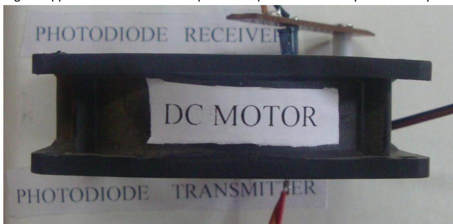
Fig 6: Setup of RPM Measurement and Control of PMDC Motor
