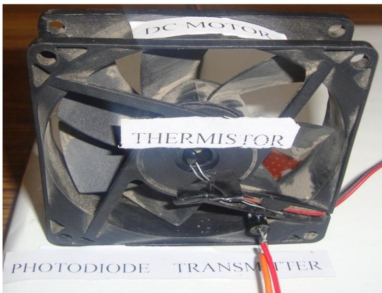
Fig 7: Setup of Online Thermal Protection of dc Motor
