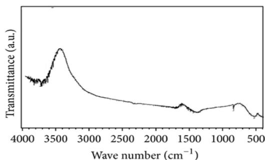
Figure 3: FTIR spectra of NLAf nanoferrites calcinated at  $750^\circ\text{C}$
