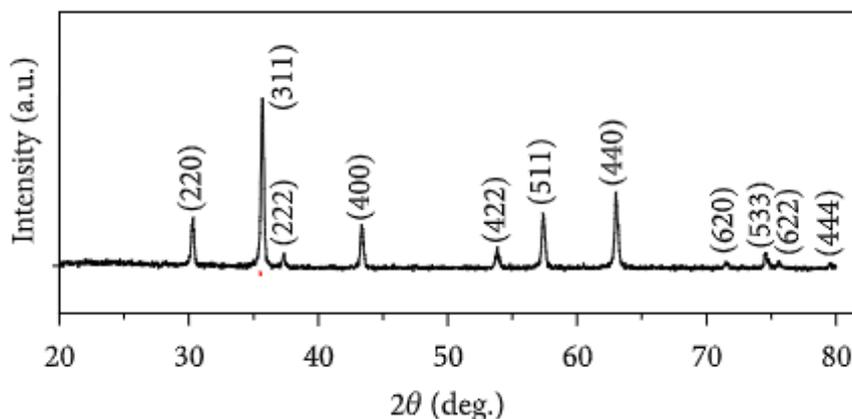
Figure 1: X-ray diffraction patterns of NLAF spinel Nanoferrites
