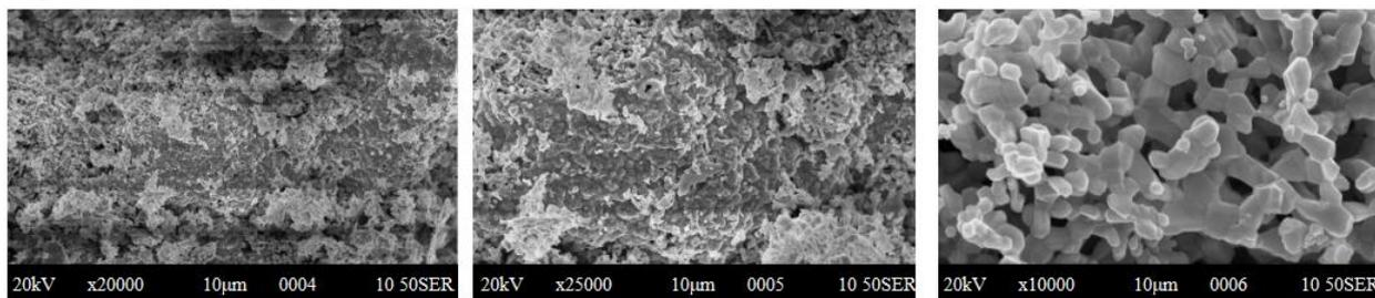
Figure 4: SEM images of NLAf nanoferrites calcinated at 750°C at different magnifications
