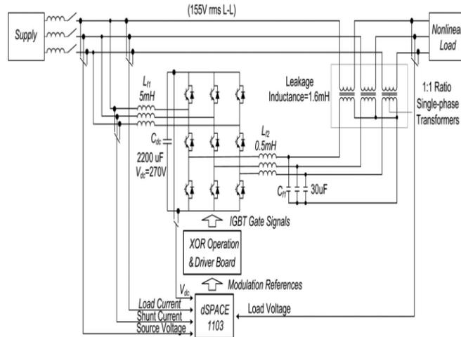
Fig4. Simulation circuit diagram of upqc
