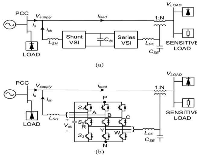
Fig. 1. Representations of (a) back-to-back and (b) nine-switch power conditioner
