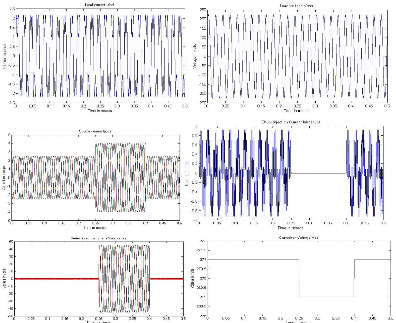
Fig5: simulation results for series injection, and load voltages during normal-sag-normal condition
