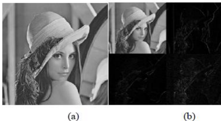
Figure 4. (a) Original image-Lena (b) Result after the first-order 2-D Haar- DWT
